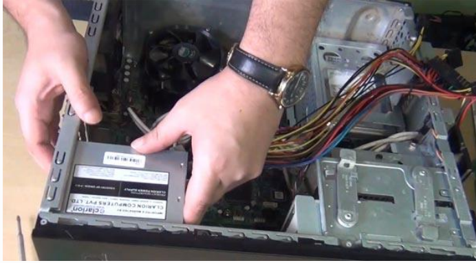
Fig: Install Power supply unit (SMPS)
